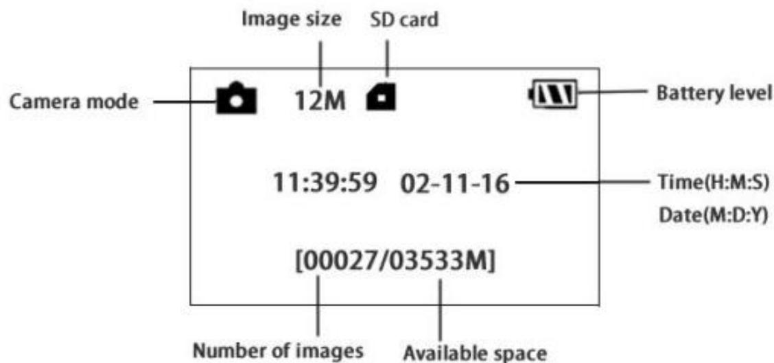
If the camera is left unattended for 20 seconds, the camera switches to “Hunting Mode”, which is the normal operation for the camera to react to motion and capture photos/videos. Before entering “Hunting Mode”, the front (red) LED light will continuously blink for approximately 10 seconds and then turn off – This a transitional delay for you to lock and mount the camera before the PIR sensor becomes active and starts taking pictures/videos.
