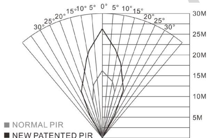
The PIR detection angle ( $\alpha$ ) is just smaller than the field of view (FOV) angle ( $\beta$ ). The advantage of this design is to reduce empty picture rate and capture most, if not all, objects in motion.
