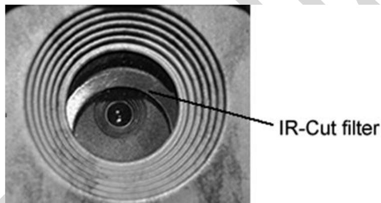
A: The camera is not broken. It's an IR-cut filter. When the camera is powered on, the IR-cut will cover the lens. Only when the camera is powered off, the IR-cut will be at a random place, sometimes covering the lens.
